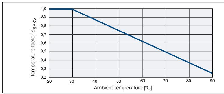
3) When coupling temperatures are higher than  $30^\circ C$ , this value must be reduced by the temperature factor.
